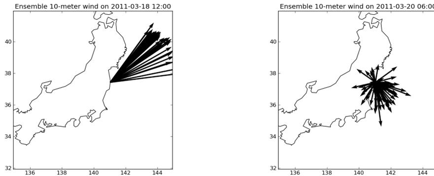
Figure 2: Illustration of uncertainties in wind forecasts, here from **TIGGE**. Each arrow corresponds to one forecast from an ensemble of simulations. The uncertainties can be very high, especially on the wind direction when the wind velocity is low.
